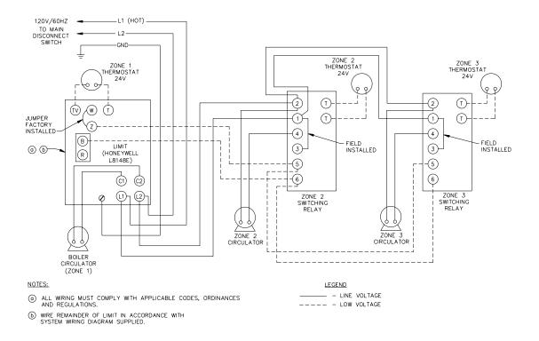
Figure 6.6: Zone Wiring with Circulators
